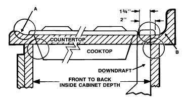
Pay special attention to the areas of potential interference highlighted above. A countertop with (A) a raised lip and/or (B) a backsplash may not allow enough flat countertop for a proper installation. Note that 2" of flat countertop is required behind cooktop and that 1-3/4" is necessary between the back edge of the cooktop and the inside of cabinet back.
